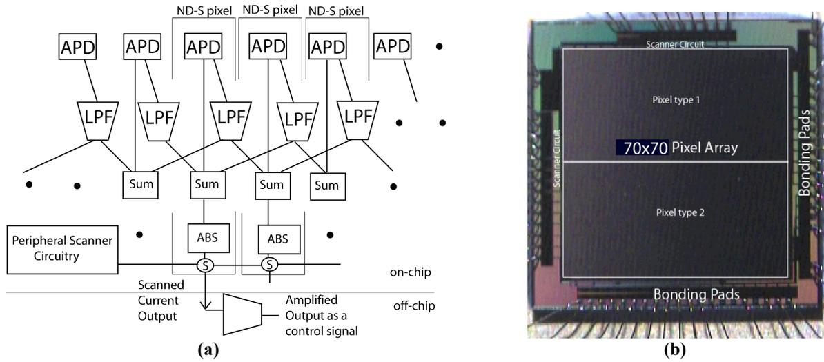
Figure 2: (a) Block diagram of the computational architecture. The output from the chip is measured by using a current-sense amplifier circuit external to the chip. (b) Photomicrograph of the integrated circuit.
