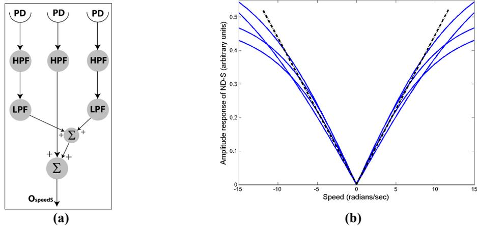
Figure 1: (a) A non-directional summation unit (ND-S). (b) Response of a ND-S unit at different spatial frequencies (solid line curves). The dotted line shows linear speed response.
